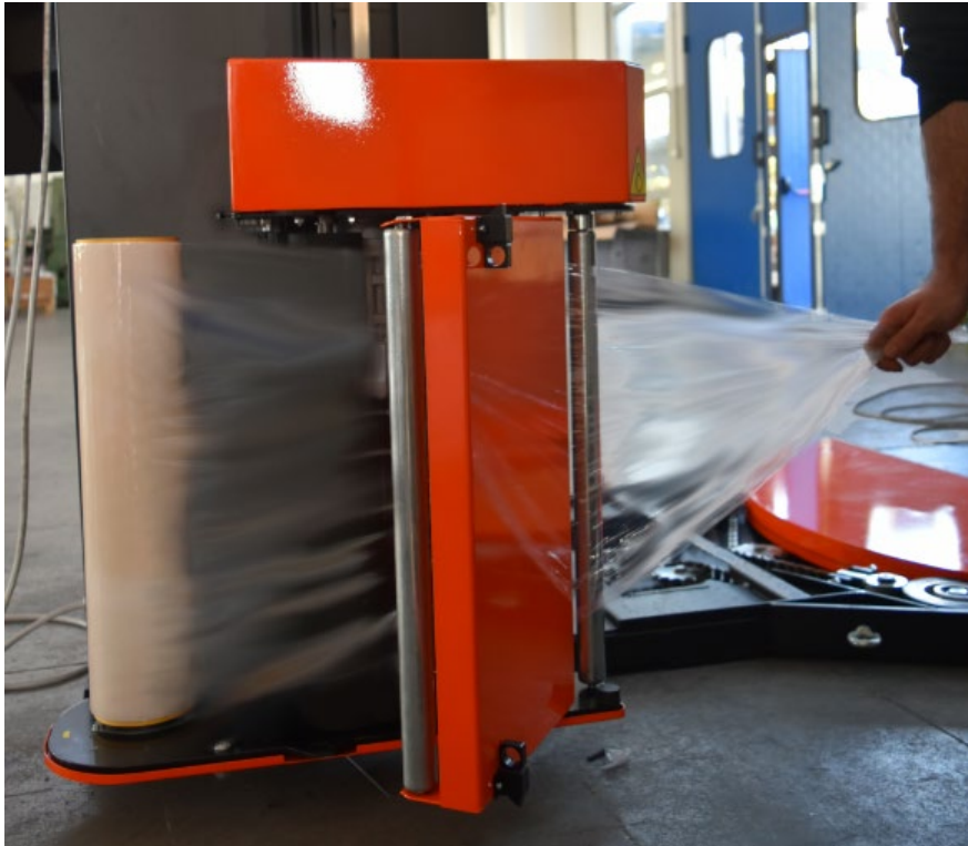
Phase 2-B: pass the film end through the carriage rollers, as shown in the picture.
