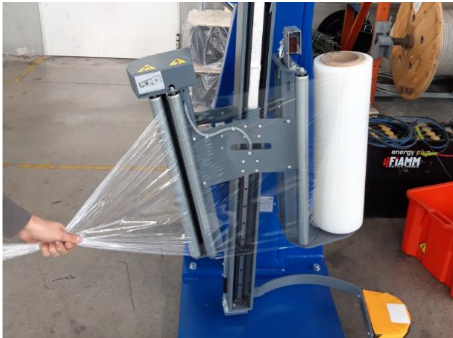
Phase 2: Pass the film end through the carriage rollers, as shown in the picture.
