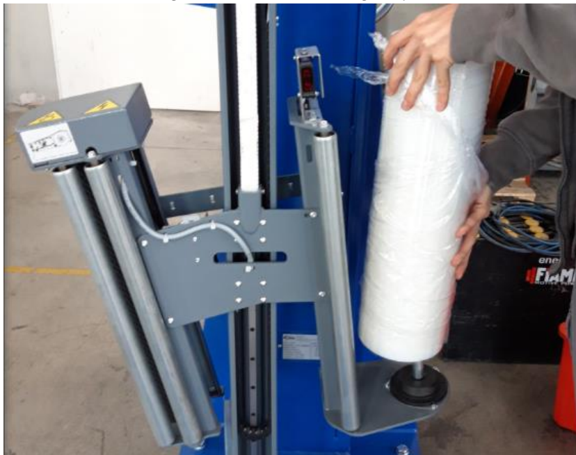
Phase 1: Insert the new film coil in the coil holder.
